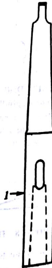
Figure 5.20 Drill socket 1. Socket body.
