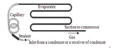
Physically the capillary tubes are hollow tubes made with drawn copper, with internal diameters ranging between 0.51 and 2 mm
