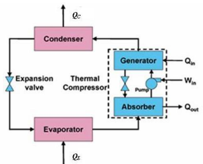
Mechanical compressor, however, is replaced by a thermal compressor which consists of absorber, solution pump, generator (or boiler) and liquid valve.
